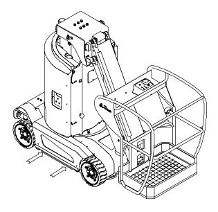
Position the forklift forks in position as the figure above.
