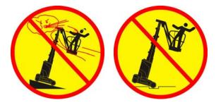
Do not use the platform controls to free a platform that is caught, snagged or otherwise prevented from normal motion by an adjacent structure. All personnel must be removed from the platform before attempting to free the platform using the ground controls.
