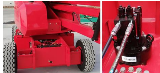
Bleeding slewing motor
