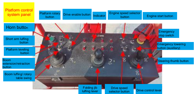
Platform control system panel
