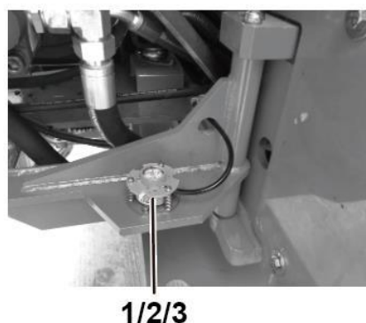
Fig. 3.79 Assembling tilt sensor
