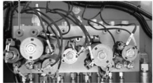
Fig. 5.9 Boom control valve set
