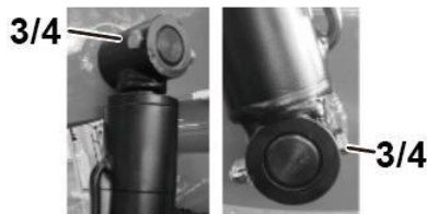
Fig. 3.35 Assembling folding jib lift cylinder
