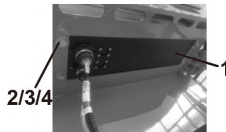
Fig. 3.7 Platform controller box
