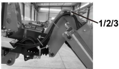
Fig. 3.17 The upper control connecting line is fixed with the flyarm valve block tubing
