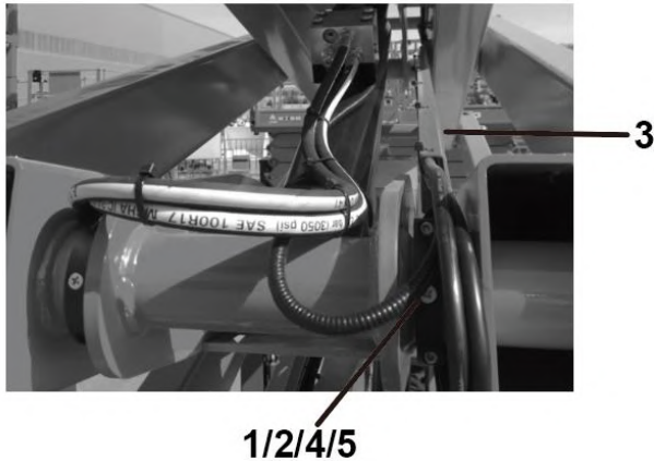
Fig. 3.27 Three-layer cable board assembly (SR1218D)
