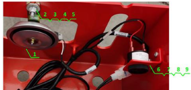
Fig. 5.3 S2632 II, S2632E II, S46 II, S46E II horns and buzzers
