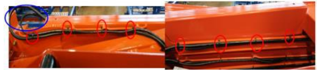
Use only the upper hole on the wiring plate for fixing
