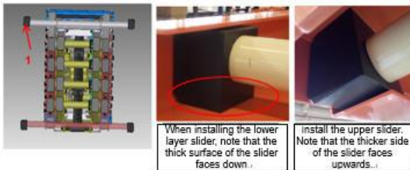
Fig. 4.70 Slider Assembly
