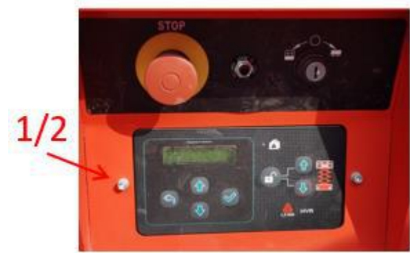
Fig. 5.21 Platform control panel
