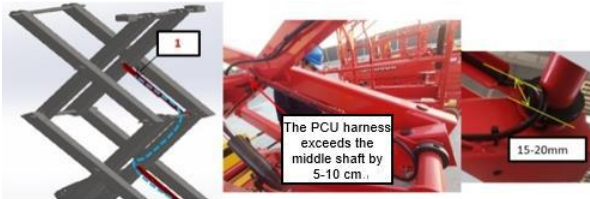
Fig. 4.29 Installation of third layer pipeline
