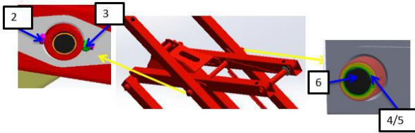
Fig. 4.27 Installation of third layer fork
