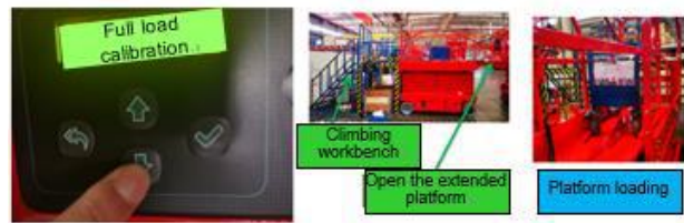
Fig. 9.16 Heavy load calibration
